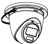
Figure 2-25 Snap Camera into Installation Plate
