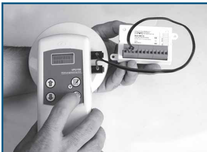
Figure 34 - Addressing modules using a VPU100
